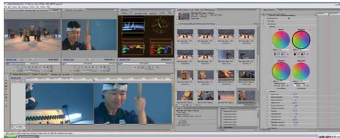
**Realtime proc amp controls** — Matrox Axio LE lets you easily adjust four proc amp controls – hue, saturation, brightness, and contrast. Hue adjusts the tint of the colors in the image, saturation adjusts the vividness, contrast adjusts the difference in luminance between the lightest and darkest areas of the image, and brightness adjusts the level of black. You can also use these controls to create special effects, such as black and white, in real time.
